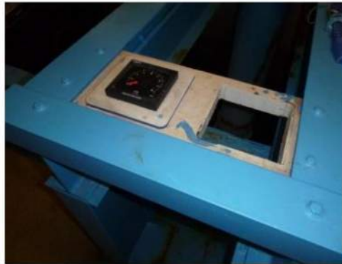
Image 44: Analog Flow Meter
