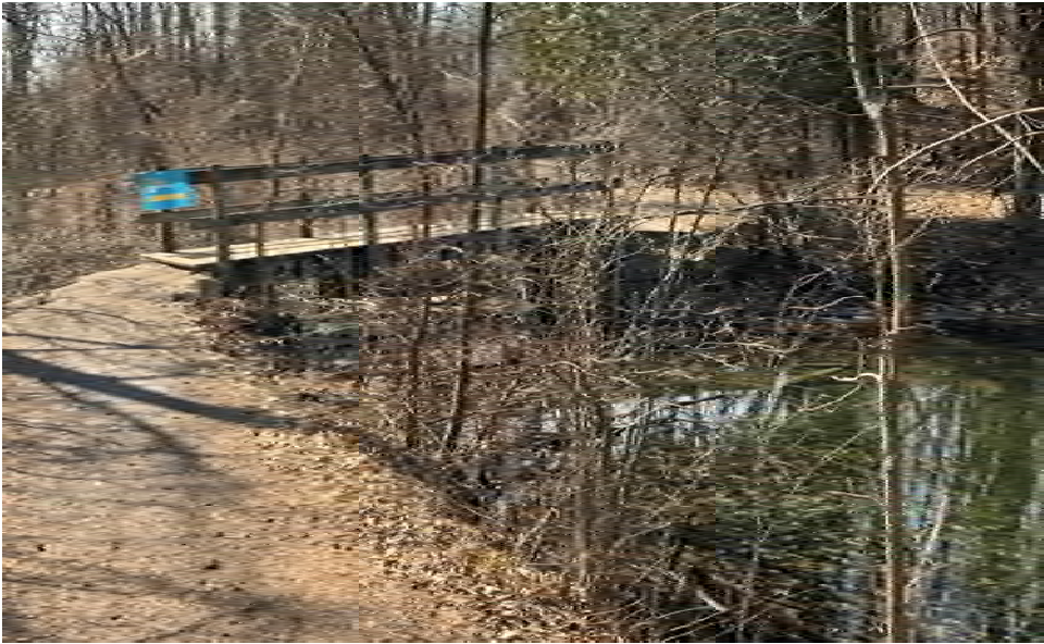
#17. (Facing Southeast): A 625 sf pond dipping platform & bridge to replace existing bridge #2. Railings to be added along South side of bridge & at the entry on & off the bridge portion of the structure. New 6' UA bench to be added.
