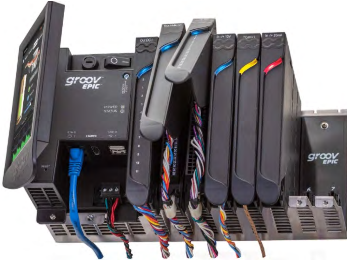
Front View of EPIC PR1 RTU and 8-Channel Chassis with I/O Modules with Display and Some I/O Modules Opened
