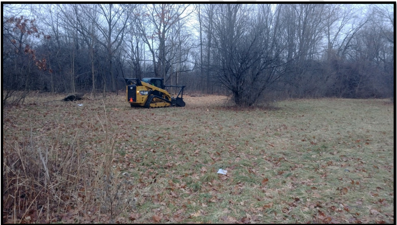
Fig. 4 Land clearing machine with Forestry Mulcher attachment removing invasive shrubs
