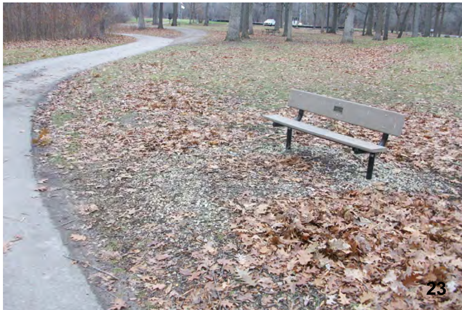
Benches to be located a minimum of 3' away from the Iron Belle Trail. Wheelchair companion seating to be provided on one side of each bench.
