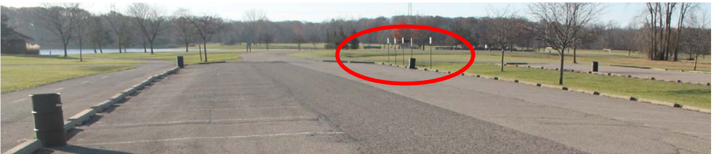
The accessible parking spaces circled above will be moved to the opposite side of the lot adjacent to the Iron Belle Trail. Four spaces will be striped for van accessibility, 2 of them will be signed for vans.
