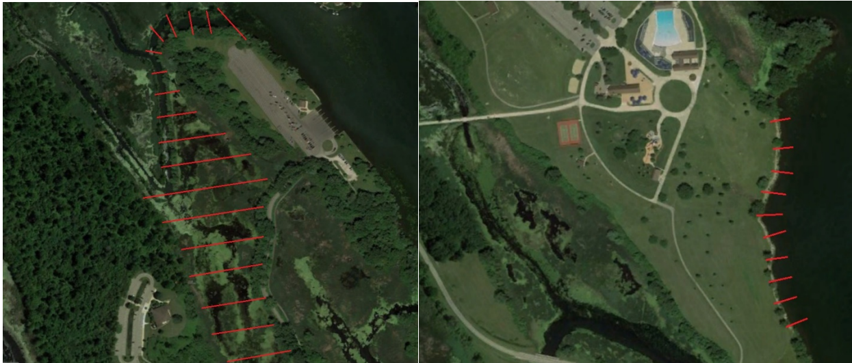
Proposed soft sediment cross-sections in the coastal marsh (left image) and connecting channels and cross-section data needed for Lake Erie shoreline (right)
