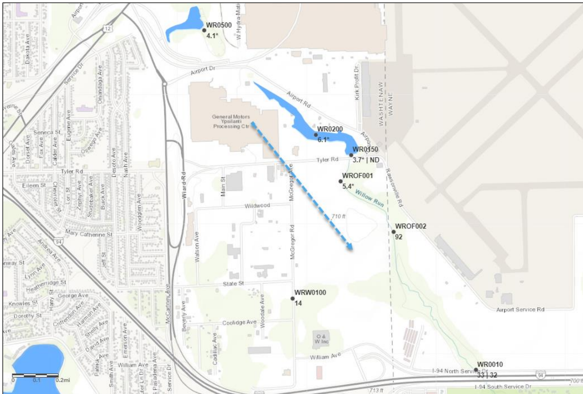
Figure 4: Sample results (PFOS ng/L) on Willow Run. Samples exceeded the HNV for PFOS at WROF002, WR0010, and WRW0100. Concentrations that were less than the reporting limit but greater than or equal to the method detection limit are marked with an asterisks (*). Concentrations that were less than the detection limit (non-detect) are displayed as "ND". Results from duplicates and replicates are shown for samples with two concentrations.
