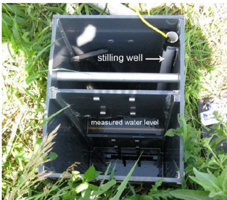
Figure 3. Outlet control box with stilling well.
